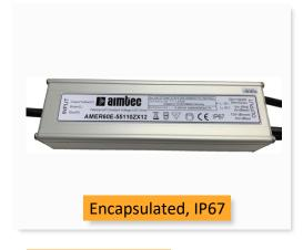
Aimtec's AMER60E-Z series is a 60W AC/DC LED driver featuring a constant current output mode and an always-on 12V auxiliary output, targeting LED lighting applications. The driver has an input voltage range from 90-305VAC and has an output voltage range of 5 to 55V at 1.1A.
