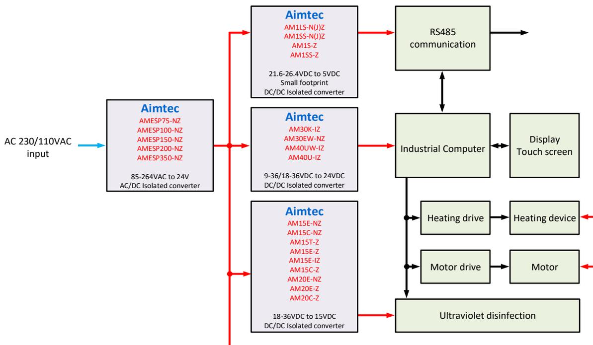
Figure 1. Automatic nucleic acid extraction instrument
