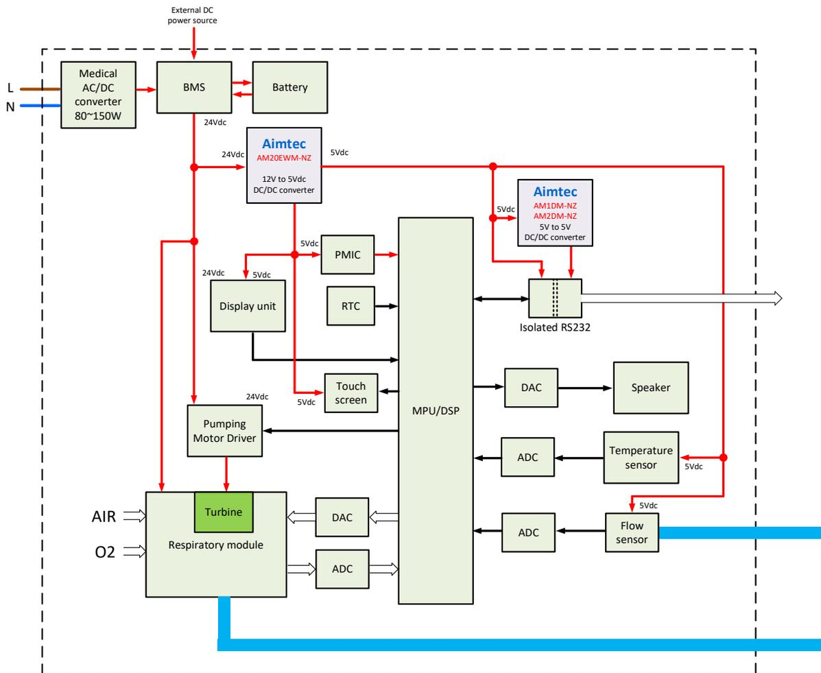
Figure 6. Transport ventilator
